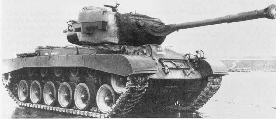
The T40 was later designated the M46 and can easily be distinguished from the M26 by the barrel bore evacuator, fender mounted mufflers and exhausts, and compensating idler wheel in front of the drive sprocket. The mufflers were eventually covered by metal shields to prevent burns to tank and maintenance crews. (Binder)
