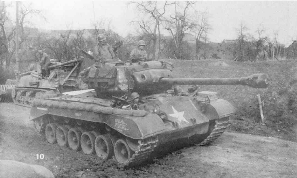
This Pershing from C Company, 19th Tank Battalion, 9th Armored Division, moves up a road between Thum and Grinnick on 1 March. The drivers' foul weather hoods are stored in the turret side rack, while the vehicle tarp is stowed alongside the starboard fender storage containers. A yellow air identification panel has been tied across the rear deck. (PAM)
