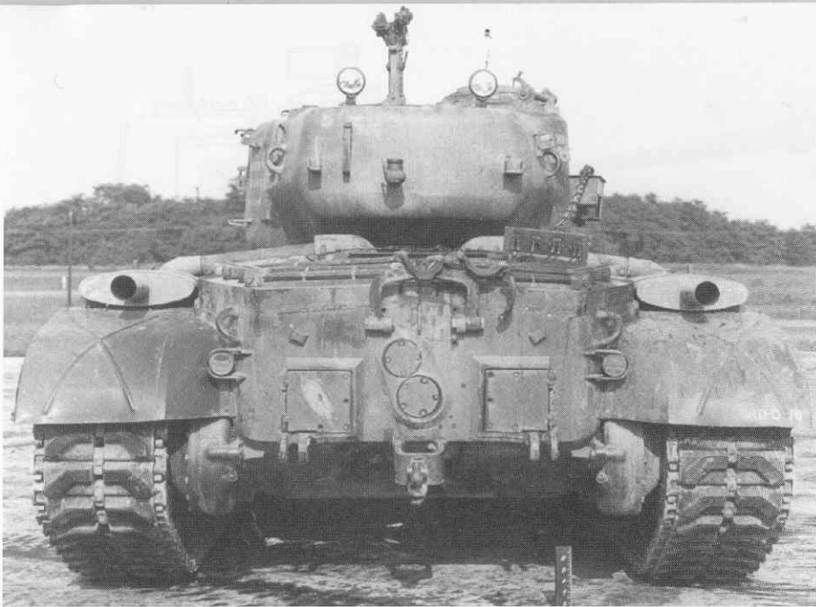
The M26E2 rear hull was also changed compared to the M26. Hinged square hatches were added to the rear plate to provide access to the new transmission. While the M26 had its exhaust nestled between the barrel travel lock arms, the new exhausts were now ducted to mufflers mounted on each fender. (Hunnicuttt)
