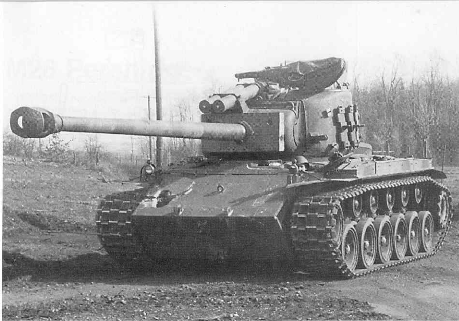
The pilot model T26E1 was fitted with the 90mm T15E1 gun. This weapon was comparable in performance to the 88mm gun mounted in the Tiger II. Additional armor was welded to the front hull and gun mantlet. Two cylinders with coiled springs were mounted atop the turret and attached to the mantlet to help compensate for the longer, heavier gun barrel. (Hunnicut)
