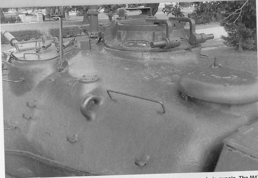
The roughly cast turret was equipped with both a loader's hatch and commander's cupola. The M47 commander's cupola was an improved version of the type used on the M46. The barrel travel lock for the commander's .50 caliber machine gun is mounted behind the loader's hatch. This location was somewhat further forward than on the M46. The ventilator/blower housing is to starboard in front of the storage box. (Author)
