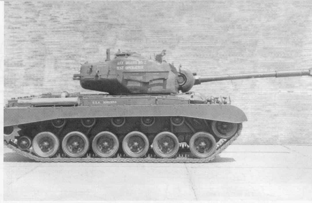
A further upgrade involved the addition of a new 90mm M3A1 gun with a bore evacuator and single baffle muzzle brake. An improved AV-1790-3 engine and CD-850-2 transmission replaced the original powertrain. A small compensating idler wheel was added between the last road wheel and drive sprocket to help prevent tracks being thrown in a turn. This model was designated the T40. (PAM)
