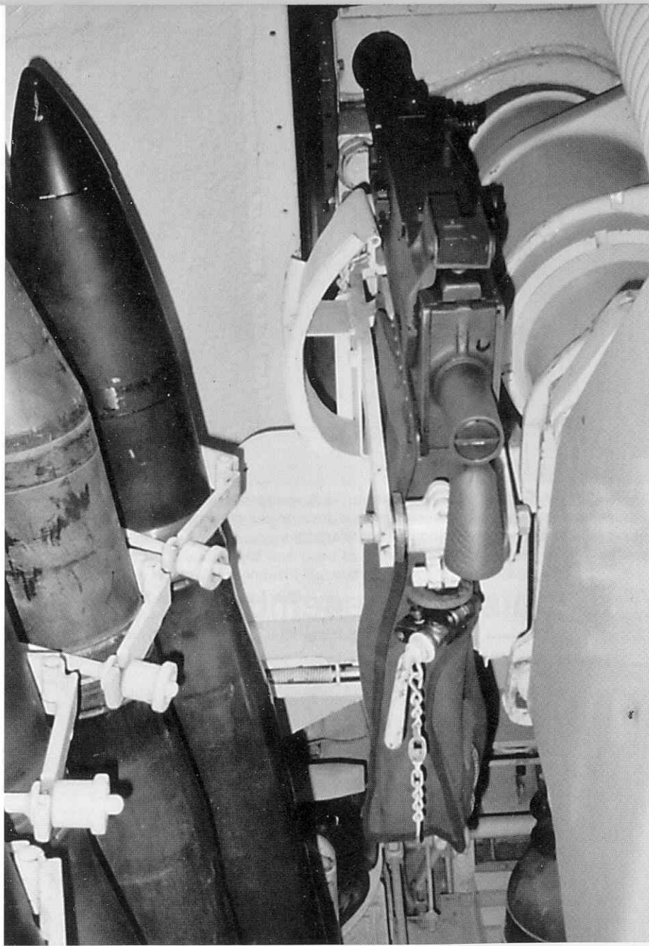
The loader's position held ten vertically mounted rounds of 90mm ammunition in the ready rack. The M26 used both armor piercing ammunition against enemy tanks and high explosive rounds against soft targets. The .30 caliber co-axial machine gun was mounted directly to port of the main gun. Spent machine gun rounds were funneled into a canvas bag fitted under the weapon. (Ward)
