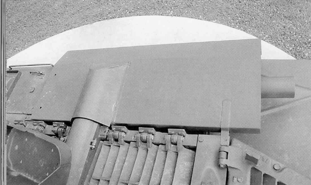
Sheet metal shields covered the M47 mufflers to prevent accidental burns from the hot surface – a carryover design element from the previous M46. A metal cover was also placed over the exhaust piping coming out of the engine. The jerry can holder at the lower left was attached to the side of the storage box. (Author)
