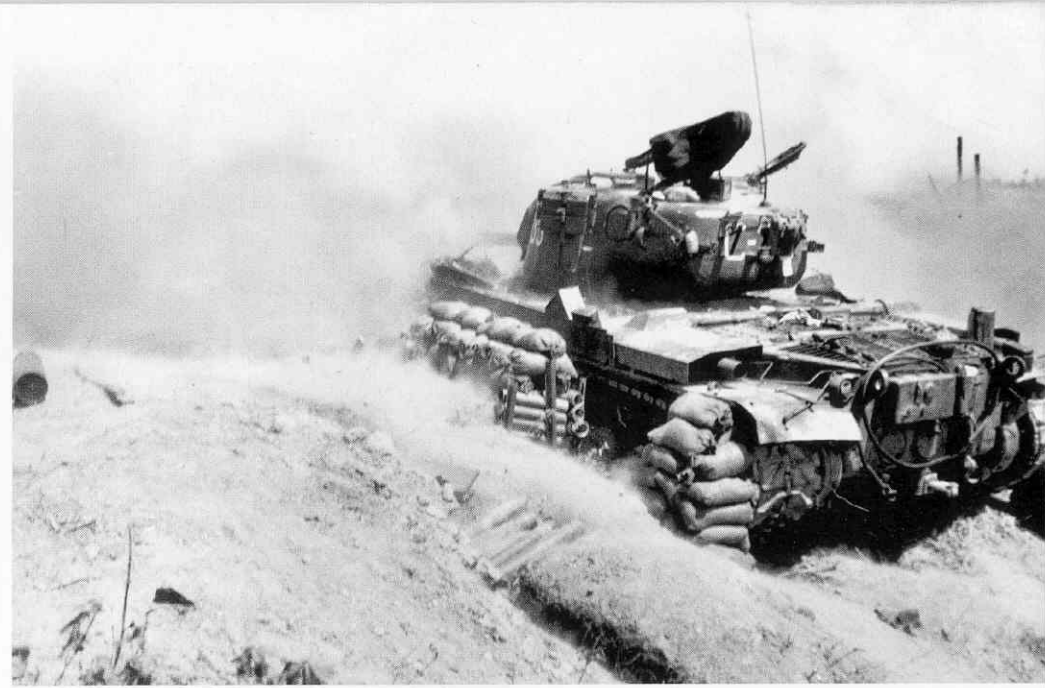
Elaborate bunkers were sometimes built around the tanks using sandbags, crates, and shell casings. This Marine M46 has just fired at an enemy bunker and the gun blast has raised a huge cloud of dust. This made it easy to spot the tank's position and sometime invited counter-battery fire from the North Korean lines. (USMC/NA)
