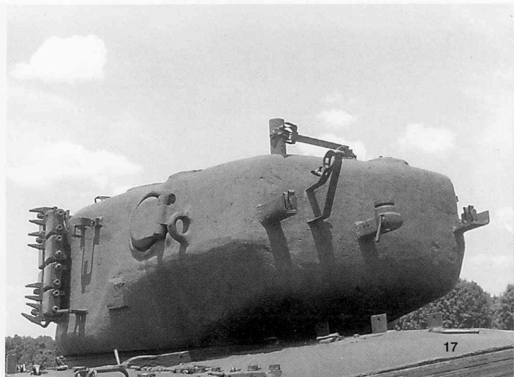
(Above) The gun mantlet was 4.5 inches (11.4 cm) thick, with three openings: one for the main gun in the center, one for the gunner's telescopic sight to starboard, and one for the co-axial .30 caliber machine gun to port. The mantlet had a rough cast appearance with the manufacturer's casting marks imbedded on the upper right portion. The 90mm M3 gun was mounted on a trunion aft of the mantlet. This weapon's elevation and depression ranged from +20° to -10°. (Author)
