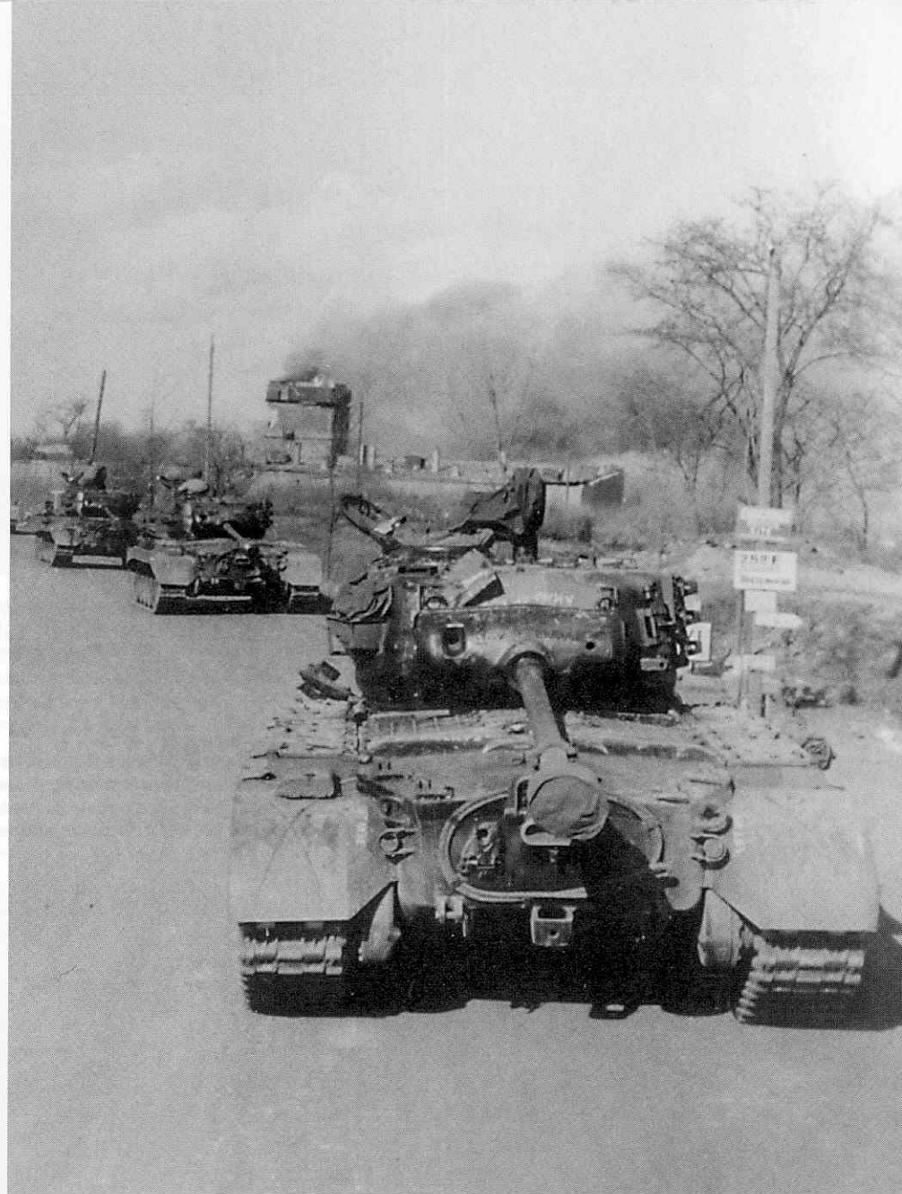
A column of T26E3s from the 2nd Armored Division moves up through Wessel, Germany toward the Rhine in the spring of 1945. The area is obviously secured as the guns are locked in the traveling position. The gun traveling lock was attached to the rear hull. A canvas cover was placed over the near tank's muzzle brake to keep moisture and dirt out of the main gun. (PAM)
