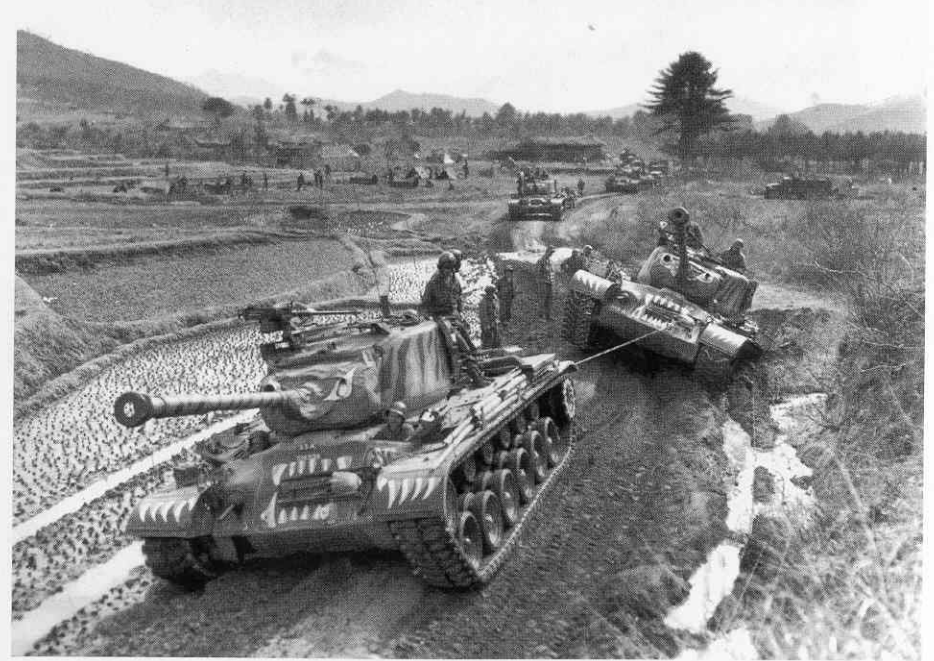
Tigers may be able to go anywhere, but some M46s are not so lucky. This 6th Battalion M46 pulls one of its fellow 'tigers' out of the mud during the spring thaw north of Chongpyong, Korea. The foreground M46 has one of the early type muffler covers, which did not extend all the way down the side of the muffler. (USA/NA)
