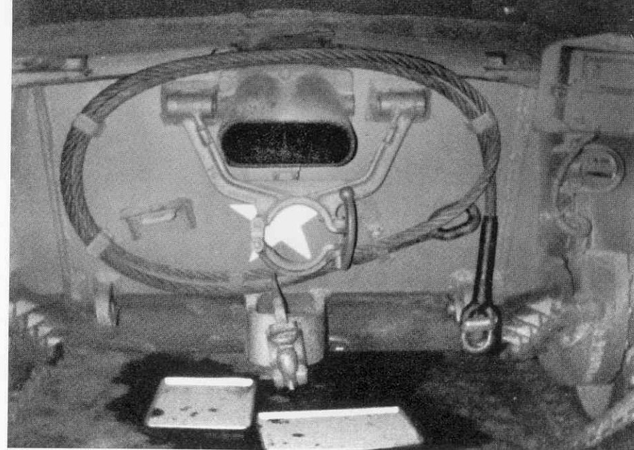
The engine exhaust pipes and barrel travel lock were mounted on the rear hull. Tow cable fittings and a mount for the tow cable were also located on the rear hull plate. The towing pintle is installed on the towing bracket. (Author)
