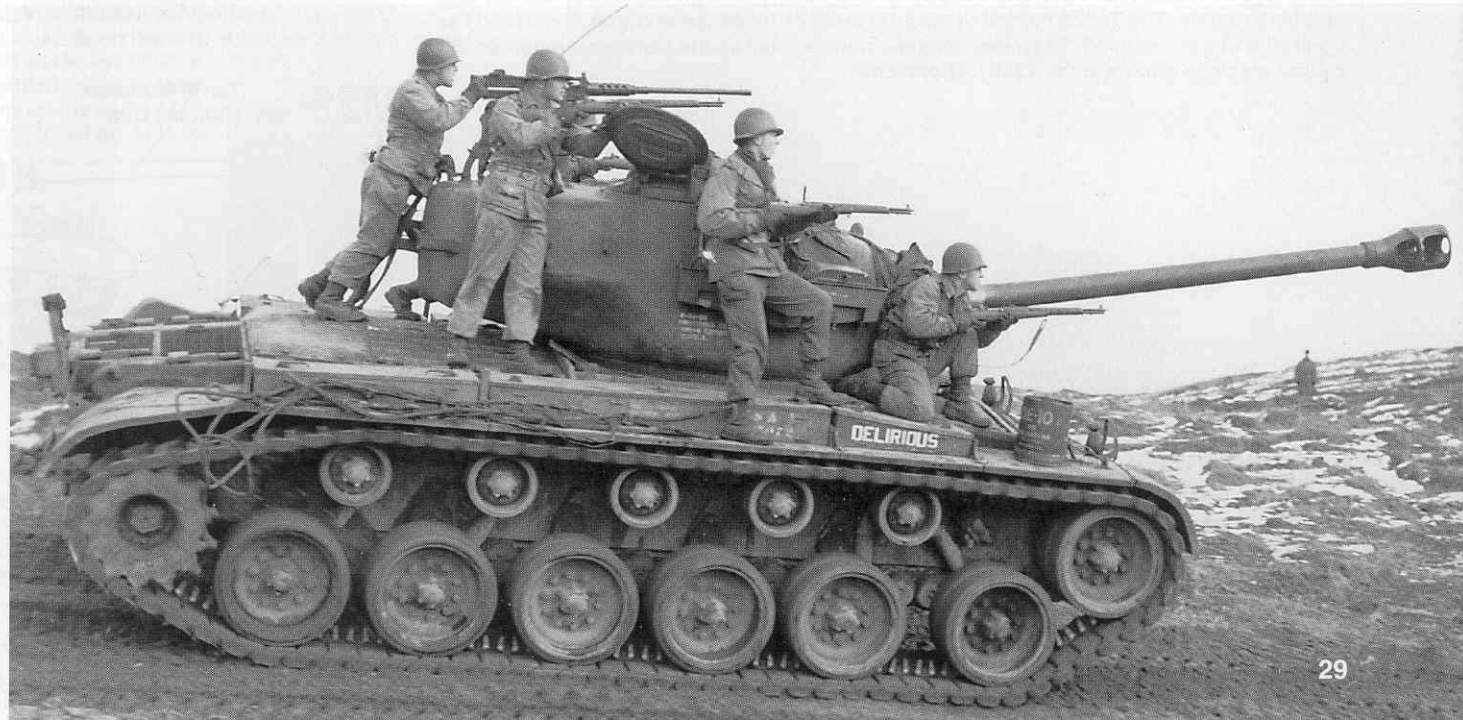
DELIRIOUS rumbles along a muddy track during training near Mainz, Germany in February of 1952. The tank was assigned to D Company, 66th Tank Battalion and was conducting training with the 42nd Armored Infantry Battalion. The loose tow cables hanging over the fender are a major safety hazard; the cable could foul the running gear or possibly drag an infantryman off the tank if it was snagged by the tracks. (USA/NA)
